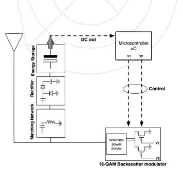
**Passive WPT WSN** Wireless powered Ĺ sensor ١ () Data transmission -() Fixed wireless power transmitter
