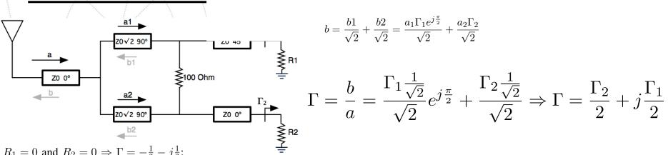
$R_1 = 0 \text{ and } R_2 = 0 \Rightarrow \Gamma = -\frac{1}{2} - j\frac{1}{2};$   $R_1 = 0 \text{ and } R_2 = \infty \Rightarrow \Gamma = \frac{1}{2} - j\frac{1}{2};$   $R_1 = \infty \text{ and } R_2 = 0 \Rightarrow \Gamma = -\frac{1}{2} + j\frac{1}{2};$  $R_1 = \infty \text{ and } R_2 = \infty \Rightarrow \Gamma = \frac{1}{2} + j\frac{1}{2}.$
